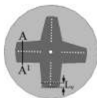
Fig. 3. Modified antenna with horizontal vias at bottom.
